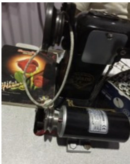
Motor that runs on solar attached to a sewing machine
